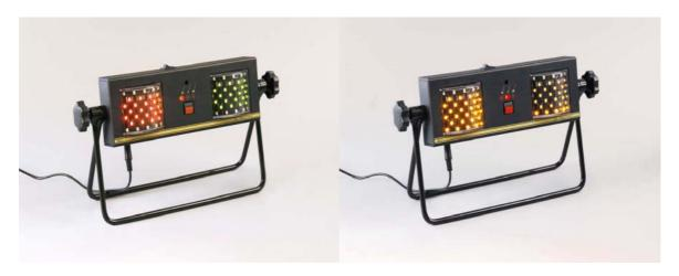
The lights used in foil and sabre to indicate antiblocking antifraud lights are located at the top of the LED displays. These lights signal a short between the fencer's weapon and his vest.
