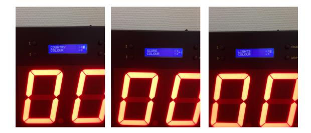
In order to transfer these parameters to the repeater, you must activate the set repeater command through the Change push button.
