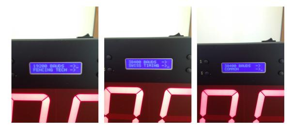
For proper command of the SG name repeaters it is mandatory to choose the Swiss Timing serial protocol with a baud rate of 38400.
